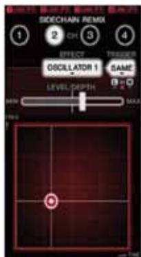
SIDECHAIN REMIX Sidechain remix uses sound on a specified channel as a trigger so that an effect can be applied to the sound on another channel.
